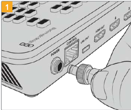
Connect power to ATEM Mini's power input using the supplied cable
