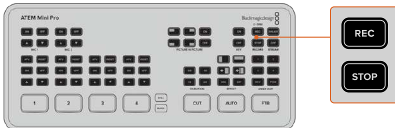
Press the record button, marked 'rec', to record your broadcast to an external drive or flash disk via USB-C
